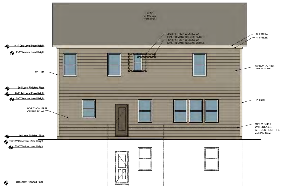
REAR ELEVATION "D" W/ 9' BSMT. SCALE: 1/8"=1'-0" (11x17" SHEET SIZE) SCALE: 1/4"=1'-0" (22x34" SHEET SIZE)
