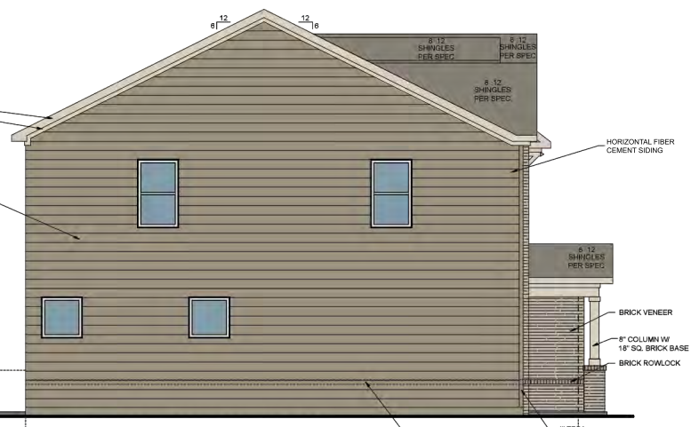
LEFT ELEVATION "D" W/ 9' BSMT. SCALE: 1/8"=1'-0" (11x17" SHEET SIZE) SCALE: 1/8"=1'-0" (22x34" SHEET SIZE)
