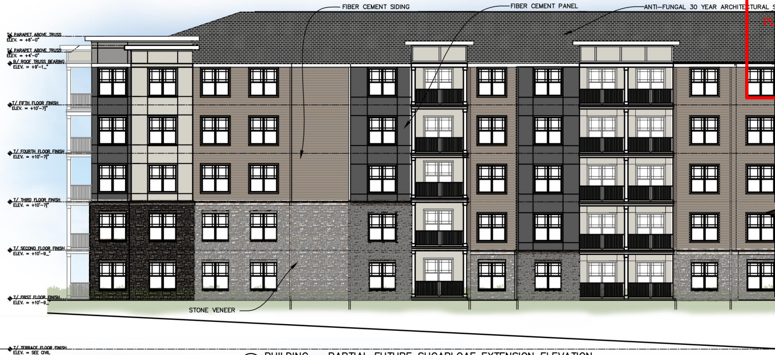
2 BUILDING - PARTIAL FUTURE SUGARLOAF EXTENSION ELEVATION 1/16" = 1'-0"
