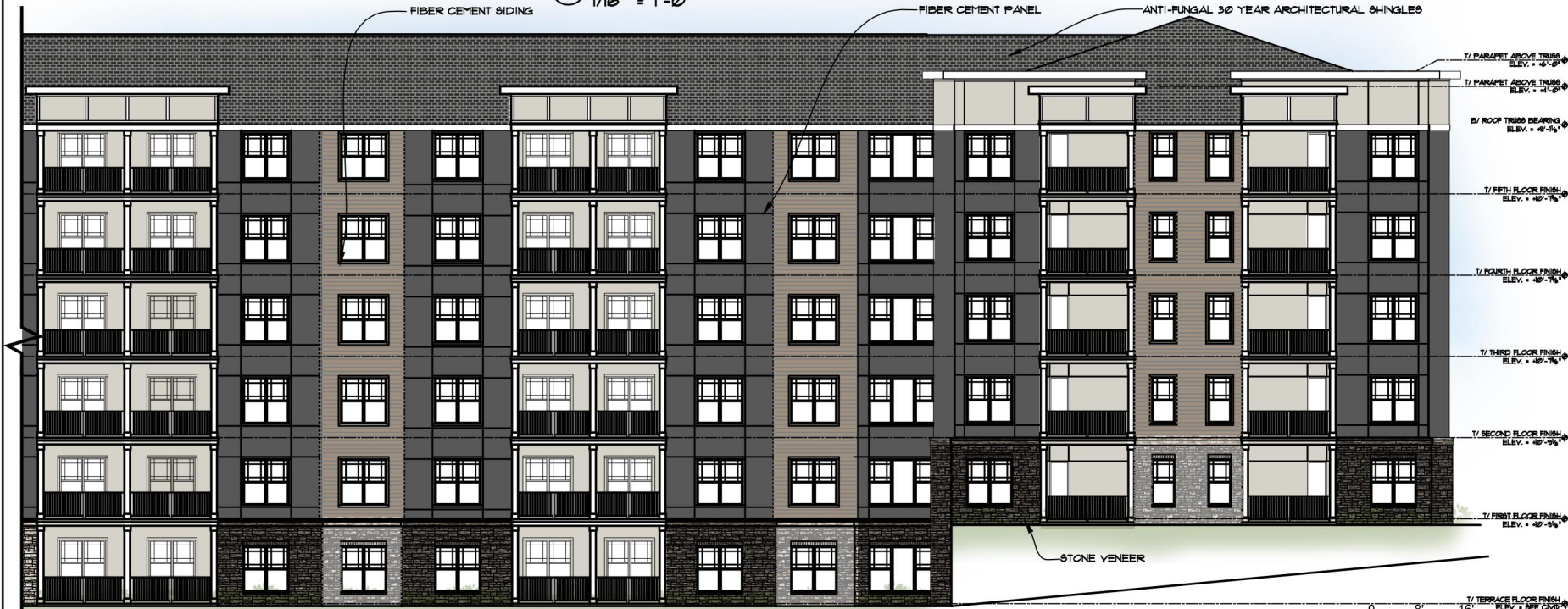
STONE VENEER 1 BUILDING - PARCIAL RIGH ELEVATION 1/16" = 1'-0"
