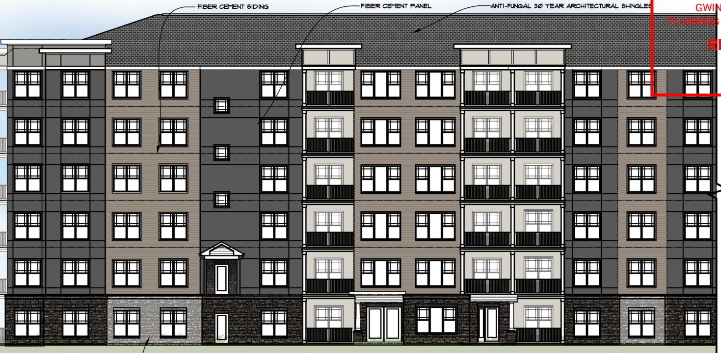
STONE VENEER 2 BUILDING - PARCIAL RIGH ELEVATION 1/16" = 1'-0"
