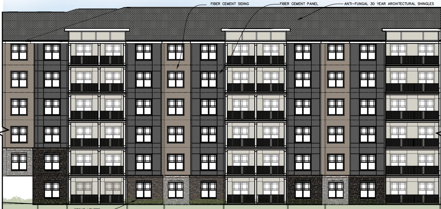
1 BUILDING - PARTIAL FUTURE SUGARLOAF EXTENSION ELEVATION 1/16" = 1'-0"
